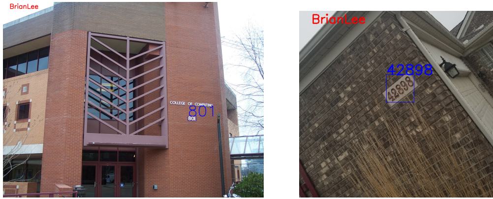
Figure 2: Positive Results. Left: Successfully detect even small scales and lots of number looking like clutters in the background. Right: Even with big rotations and lots of brick clutter in the background, correctly classifies, filters, and combines numbers.
